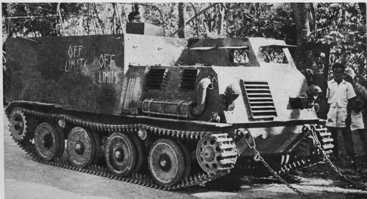
Latest personnel carrier improves on earlier Japanese models, will seat 24 men. It is armored on all sides, fully tracked and powered
